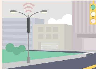
Small cells are just like the name implies – short range cell sites used to complement macro cell towers in a smaller geographic area ranging from a few hundred feet to upwards of 1,000 feet. These lower power antennas enhance capacity in high traffic areas, dense urban areas, suburban neighborhoods, and more. Small cells use small radios and a single antenna placed on existing structures including utility poles and street lights.
