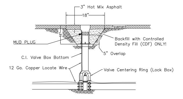
TYLER CAST IRON VALVE BOX 6855 HD, WITH NO FLIP "WATER" HEAVY LID,  $16" \times 6 \ 1/8"$  ID TO SLIP OVER C.I. VALVE BOX BOTTOM SECTION.
