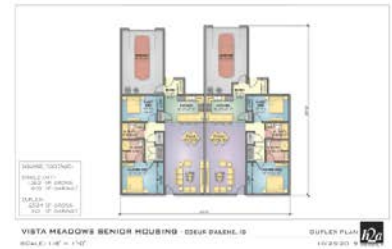
4 LOT TYPE 1 - DUPLEX - 1 STORY TYPICAL FLOOR PLAN
