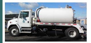
"Tank Truck" cleans the City sewer line by using 2000 gallons of water to flush the line.
