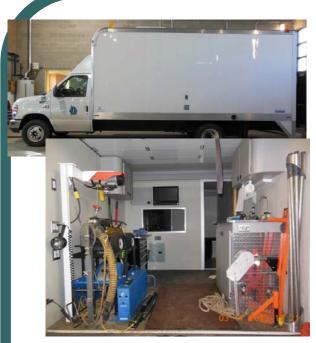
Inside the "TV Van," is a mobile office with equipment that has the capability of taking video of sewer line between 6"-36" in diameter. As video is recorded, it can then be transferred to disc for further viewing or archival.
