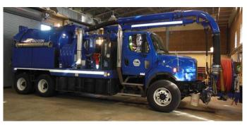
"Big Blue" Jet Truck– like the "Little Jet, Big Blue" uses hydraulic water pressure (2000 psi) to clean City Sewer lines. The difference between the two is, "Big Blue" also has the ability to vacuum debris out of the sewer line.
