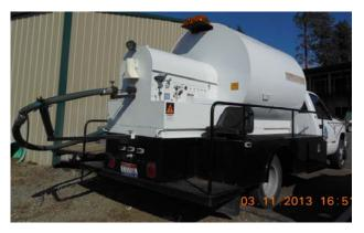
The "Rod Truck" is used in emergency situations when a line is clogged and needs a root cut or debris cut through in order to open the sewer line to increase flow through the line.
