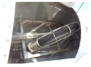
1000' Rod. The rod spool is controlled by the operator and can be moved in and out while rotating (clockwise or counter clockwise).
