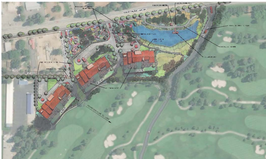
Figure 4 Concept site plan showing the buildings setback from the street and extensively landscaped garden buffering.
